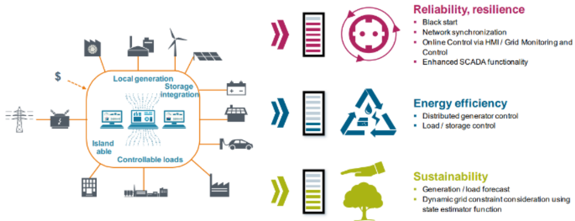
Fig. 1. Comprehensive model of a microgrid system and its key functional advantages (source: author's development)
