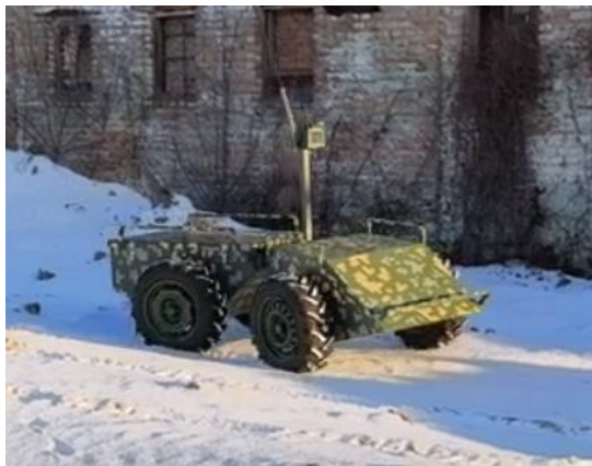
Fig. 2. UGV testing in winter conditions at -15^{\circ} C
