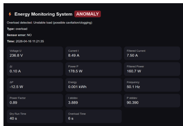
Fig. 2. User interface of energy consumption monitoring module
