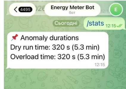
Fig. 5. Anomalous operation statistics provided via the Telegram bot
